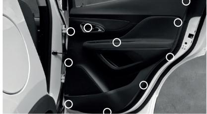
Usually the clips/screws are placed by the white marks. This could vary depending on the vehicle.
