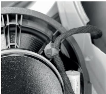
Install the speaker to the door by using the OEM M7 screw. Make sure the speaker is properly mounted and fits nicely.
