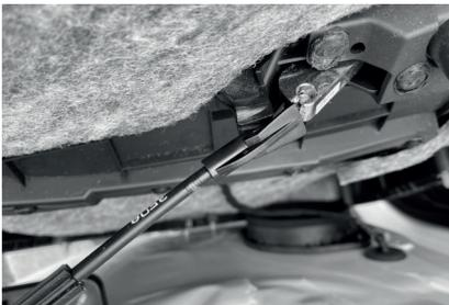
Disconnect electrical connections for the window control panel
