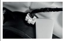
Remove the speaker by unscrewing the M10 or PH2 screws.
