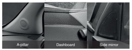
Start by removing the tweeter covers. Use plastic pry tools and be careful. The clips can be hard to remove. Take it easy and use minimal force. The instructions below show how to remove the dashboard tweeter.
