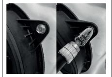
Use the pry tool to release the speaker from the door.
