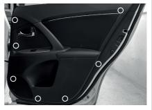
Usually the clips/screws are placed by the white marks. This could vary depending on the vehicle.
