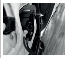
Disconnect electrical connections for the window control panel and door lights.
