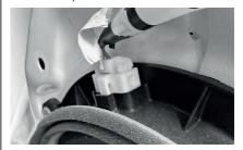
Remove the speaker by unscrewing the M10 or PH2 screws.
